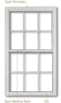
The Air Leakage (AL) rating pertains to air infiltration that occurs through the window unit itself. It is expressed as the equivalent cubic feet of air passing through a square foot of window area per minute. Air leakage typically may occur through the window assembly components, such as the sash perimeter, sash meeting rails and sill.
